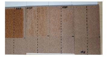
Despite all the measures, the paint system will weather over time depending on the load. One must reckon with the loss of sheen and the change in color, depending on the load. The paint structure can be overpainted, and the same material can be used to renew the weathered surfaces.
