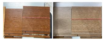
On the next picture you can see the effect of the built-in light stabilizer. The parts were tested in QUV-B 313 nm device. On the left is the zero sample without light stabilizer, on the right are the samples with 1%, 2% and 3% light stabilizer. It can also be seen that half of the part that was primed with the RBP had somewhat better durability.
