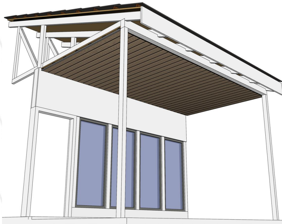
ISOMETRIC VIEW SIDING BOARD ON SOFFIT
