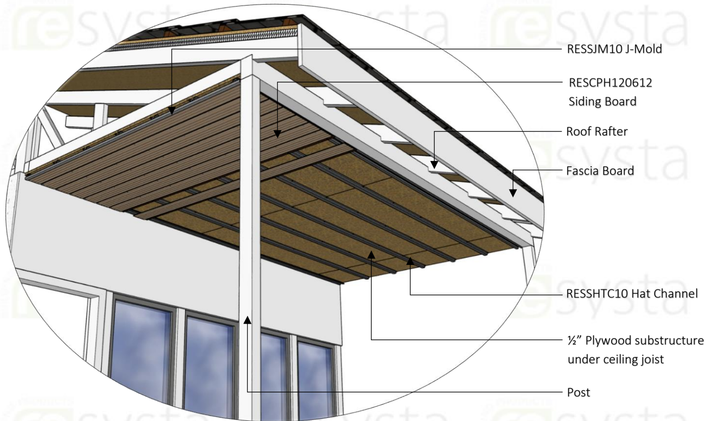
ISOMETRIC VIEW SIDING BOARD ON SOFFIT
