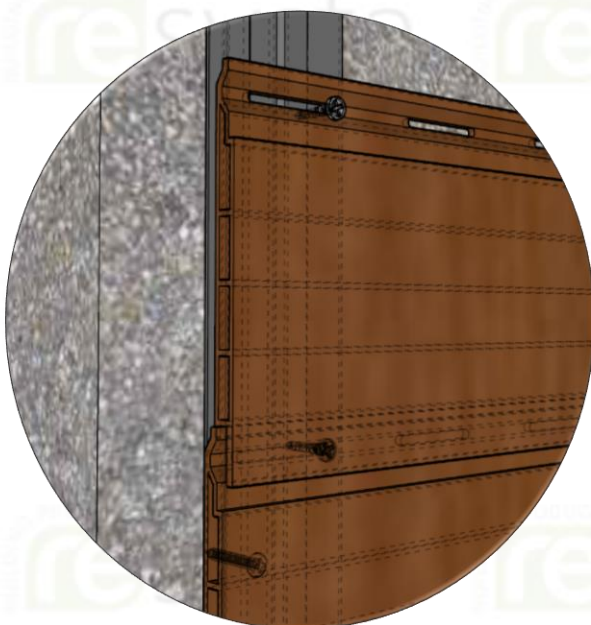
ISOMETRIC DETAIL RESYSTA HORIZONTAL SIDING
