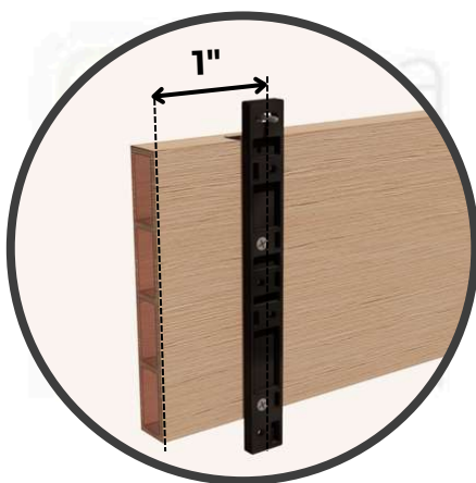
REAR ISOMETRIC VIEW HORIZONTAL WALL CLADDING DETAILS
